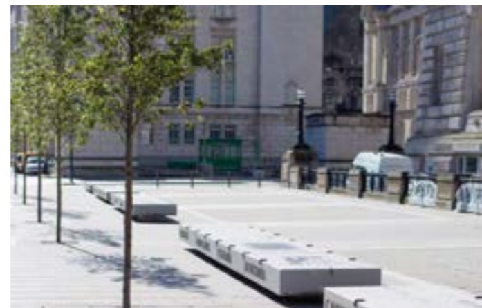
TREES AND BENCHES WILL PROVIDE AN ADDITIONAL LAYER OF PROTECTION AND DEMARCATVE VEHICULAR RUNNING ROUTES
