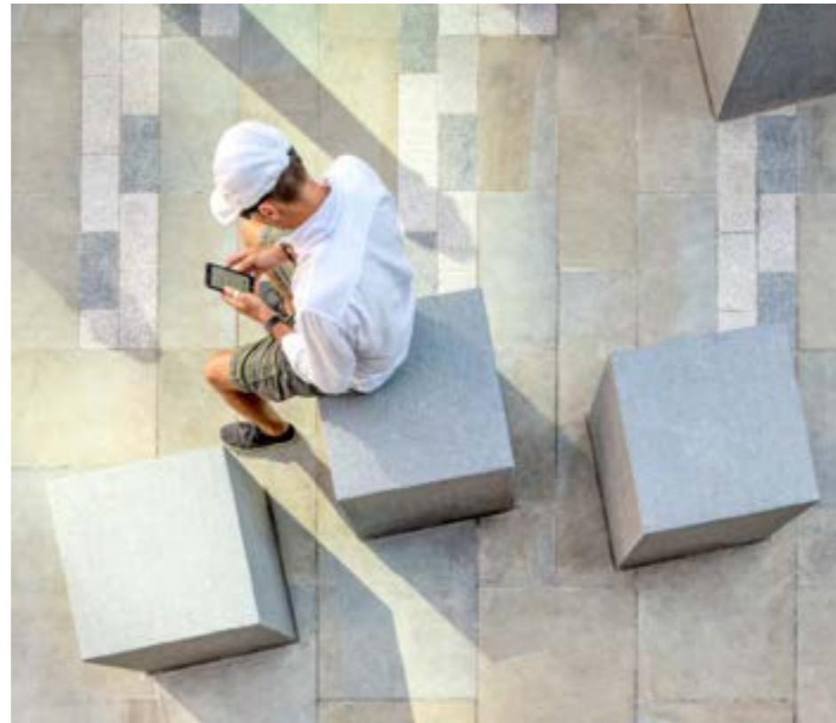
SOLID STONE SEATING CAN DOUBLE AS HOSTILE VEHICLE MITIGATION
